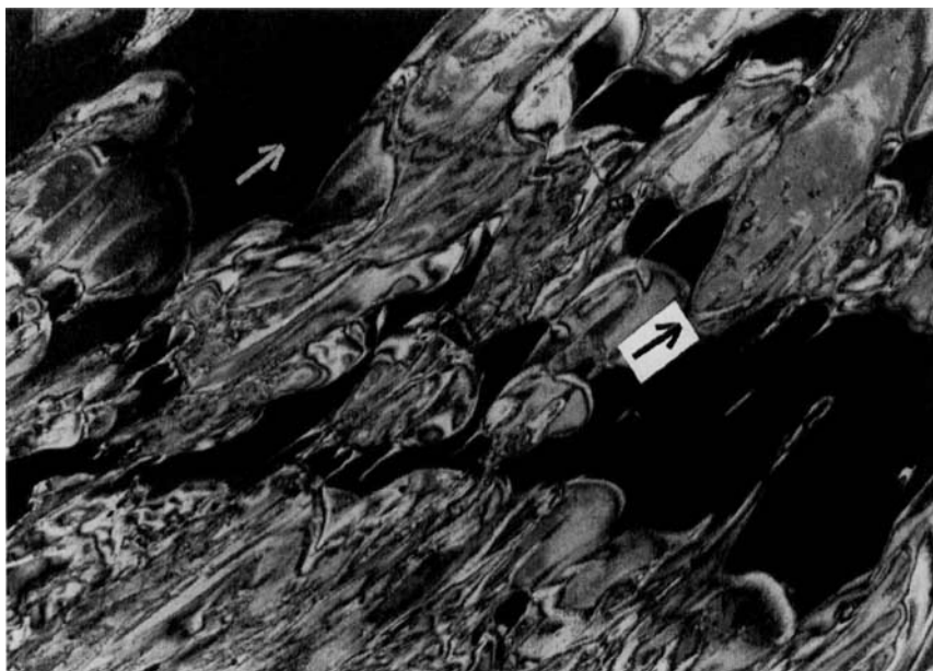
FIGURE 9 Shear-crystallised sample of the polyester of isophthalic acid and BHHBP, left on NaCl disk after shearing in the isotropic state at 140°C. The sample was mostly unoriented (white arrow), but there were oriented regions (black arrow) from which the polarised IR measurements in Figure 8c were made. Shear direction is at 45° to polar axes. (See Color Plate V).
